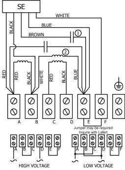
**To Change Direction of Rotation, Switch Lead "A" with Lead "C"** DVE Motors are designed for high starting torque applications. DVE motors feature capacitor start and run making them suitable for most applications (i.e. Gearboxes, pumps, and machine tools).
