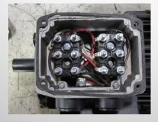
Interior view of terminal box with two terminal blocks
