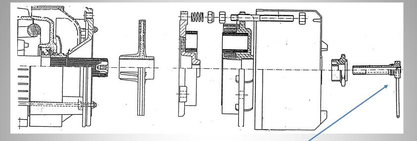
These brake motors are supplied with a manual release key to allow the brake to be disabled without applying power.
