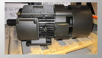
AAF132 frame with separate brake terminal box
